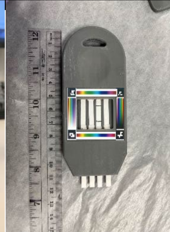
Complete sensor unit with case. Left: case only (3D-printed from synthetic resin), Right: the complete sensor inside the case
